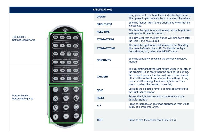
Note: To switch from motion sensor mode to dimmer mode, long press the ON/OFF button until only the BRIGHTNESS option lights up. If all options light up, long press again. Then use the -/+ buttons to adjust the brightness.
