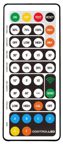
Select the desired settings (TRIM-LEVEL, SENSITIVITY, HOLD TIME, STANDBY DIM, STANDBY TIME & PHOTOCELL) or a pre-set Mode and press SEND.
