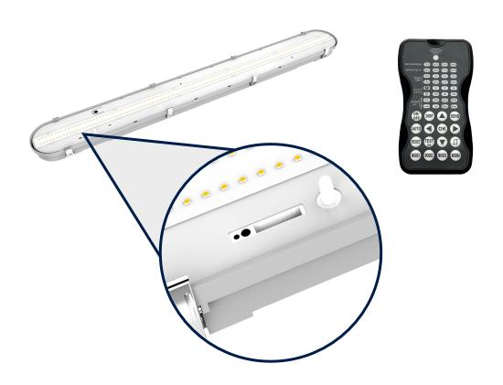
The installer can adjust the brightness of the fixture, hold time, and daylight settings using the dip switches during installation, and via remote control after installation.
