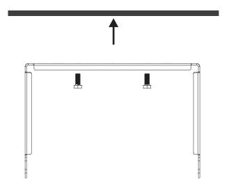
2 Secure power supply box to bracket with provided screws.
