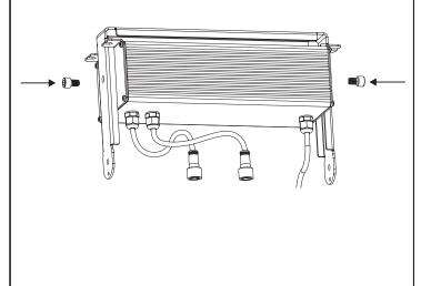
3 Secure LED fixture onto bracket with provided self-locking fastner and screw. Connect power input wires with corresponding black/white/green wires using attached connector at the end of the wires.
