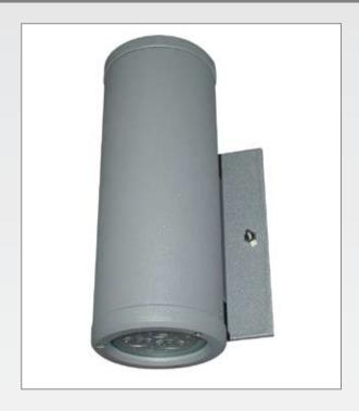
**LAMP** Takes two high power MR16 LED lamps. Each MR16 LED lamp has three 1.2 watt LED lamps with a 30 degree beam spread. Available in white, red, blue, yellow or green. Lamps included.
