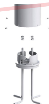
CUSTOM DESIGNED TWIST LOCK MECHANISM
