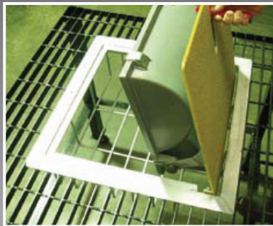
The light is attached to the underside of the hatch top plate and is revealed when the hatch is opened. Once fully opened, it stays open with its own weight.
